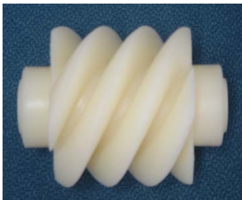
(b) Male rotor by 4 axis machining
