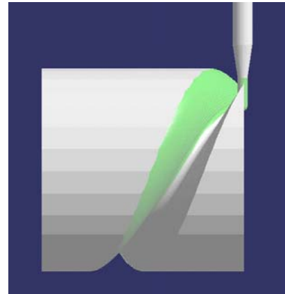
Fig. 11 Roughing the toolpath of the rotor
