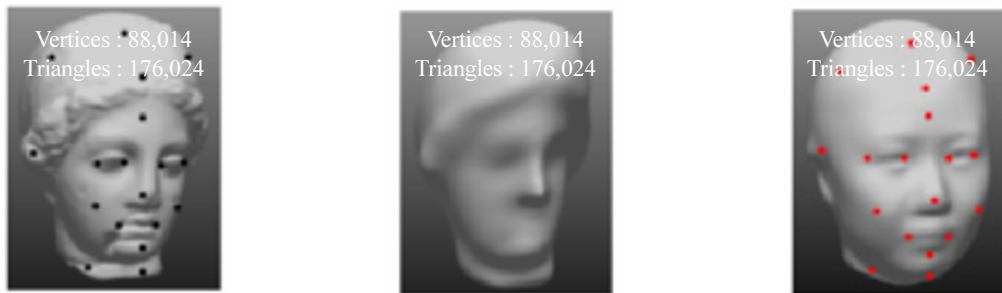
(a) Igea model (original template mesh) (b) deformed and smoothed template mesh (c) final mapped template mesh
