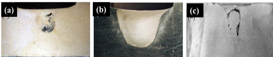
Fig. 20 Macrostructure of the SZ region. a Probe without threads, b Probe with threads, c Probe with threads along three flutes [126]
