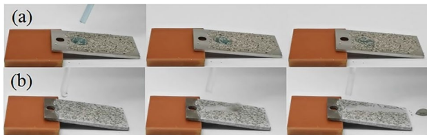
Fig. 13 Self-cleaning properties of magnesium alloy substrate a and superhydrophobic HA coating b for solid contaminants
