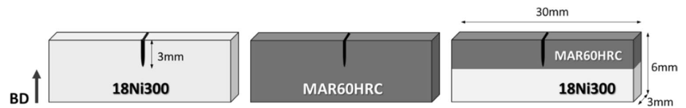
Fig. 2 Schematic of the samples prepared for fracture toughness tests
