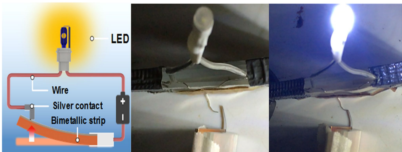
Fig. 13 A simple electrical circuit activated by the printed bimetallic strip is shown schematically and in pictures (reproduced with permission from ref. [115], under the terms of the Creative Commons CC BY license.)
