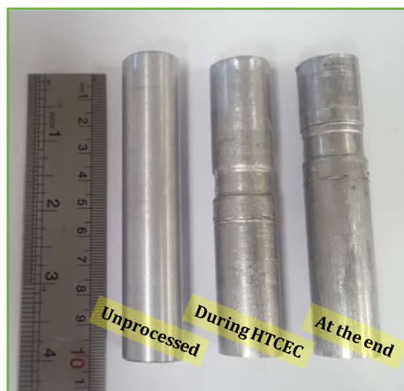
Fig. 3 The pictures of the unprocessed tube and the HTCEC processed tubes
