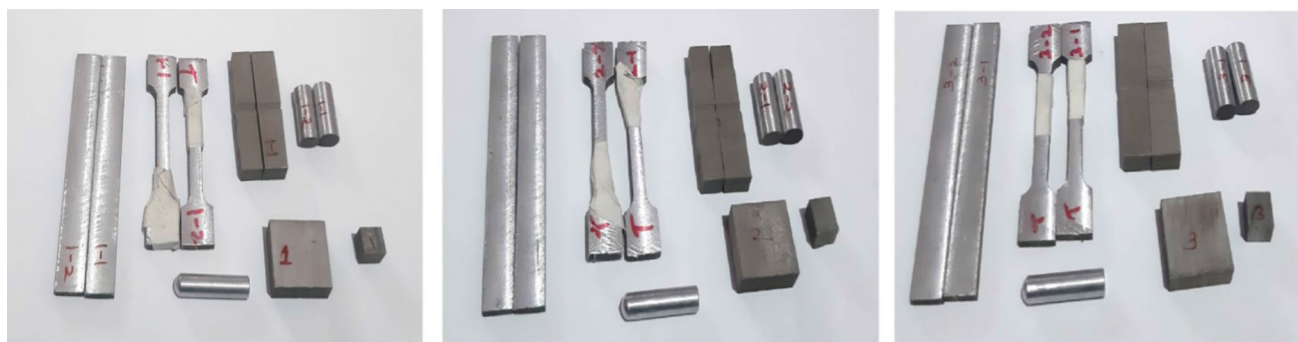
Fig. 2 \text{Si}_3\text{N}_4 reinforced composites prepared and characterized as per ASTM standards
