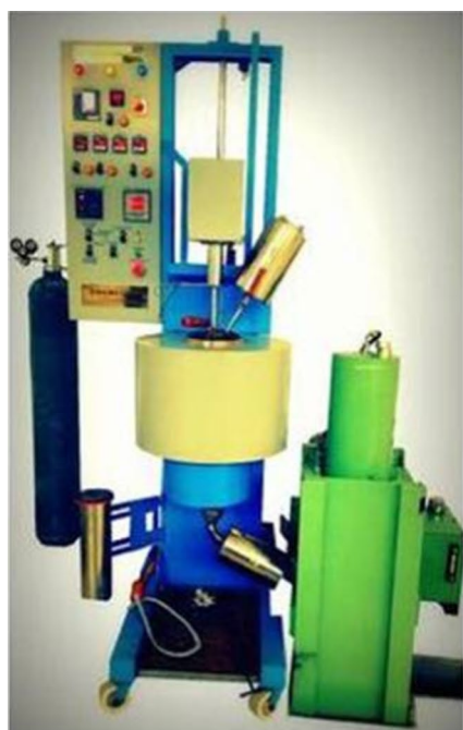
(a) Squeeze casting Setup used for synthesis of Silicon nitride reinforced aluminium composites.
