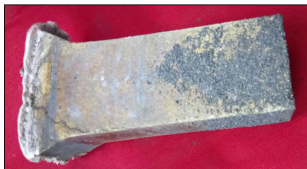
Fig. 1 Cast ingot taken from mould
