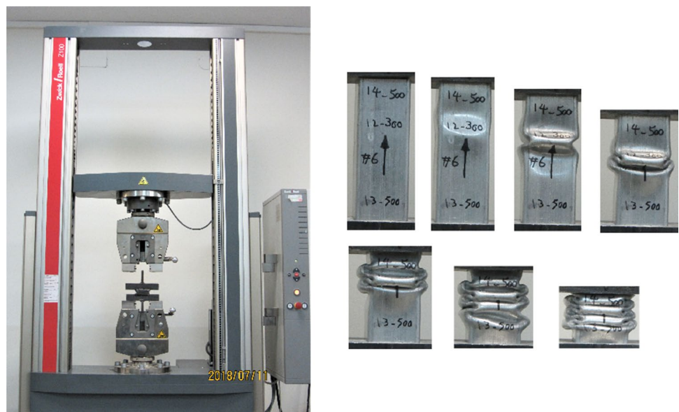
Fig. 1 Quasi-static test setup and FFT deformation mode, a universal test apparatus, b undeformed FFT, c–h deformed FFT with 10 to 60 percent strain
