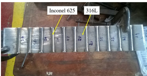
Fig. 3 Typical appearance of the clad bead
