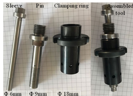
Fig. 2 Welding tool of the RFSSW
