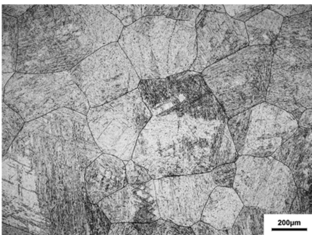
Fig. 1. Austenite microstructure after reheating at 1200 °C and 5 min soaking.
