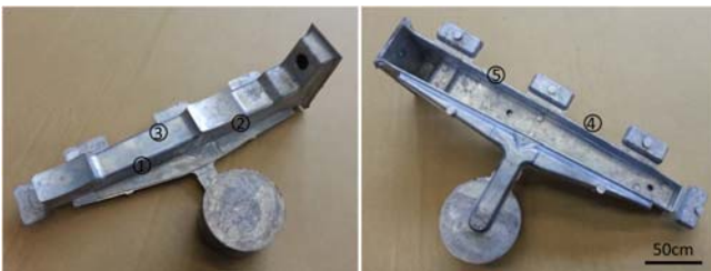
Fig. 1. The photos showing the casting structure with runner, overflow and biscuit for the evaluation of reproducibility.
