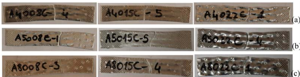
Fig. 6. Propagations of fracture in tensile specimens. (a) 0.8-1.5- and 2.2-mm bulge height of 0.4-mm- thick sheet, (b) 0.8-1.5- and 2.2-mm bulge height of 0.5-mm- thick sheet, and (c) 0.8-1.5- and 2.2-mm bulge height of 0.8-mm- thick sheet.
