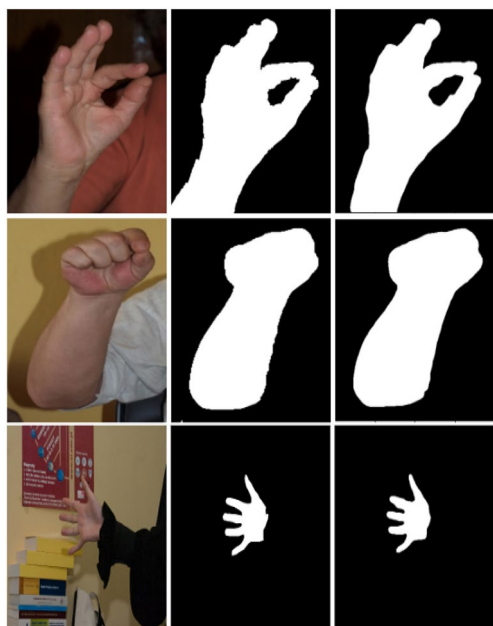
Fig. 12 Semantic segmentation outputs for HGR dataset: 1 st column shows the gesture images, 2 nd column shows the segmented masks obtained by Kawulok et al. (2014), 3 rd column shows the segmented masks obtained through attention-based UNet (our method)
