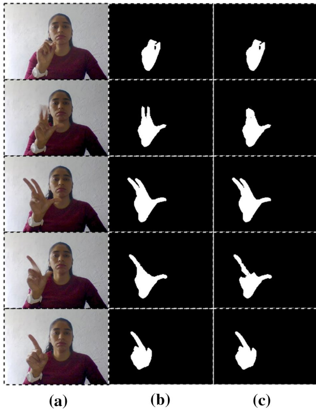
Fig. 14 Semantic segmentation output for a few dynamic gesture frames from IPN hand dataset: a shows the gesture images, b ground truths, and c shows the corresponding segmented masks obtained by our method
