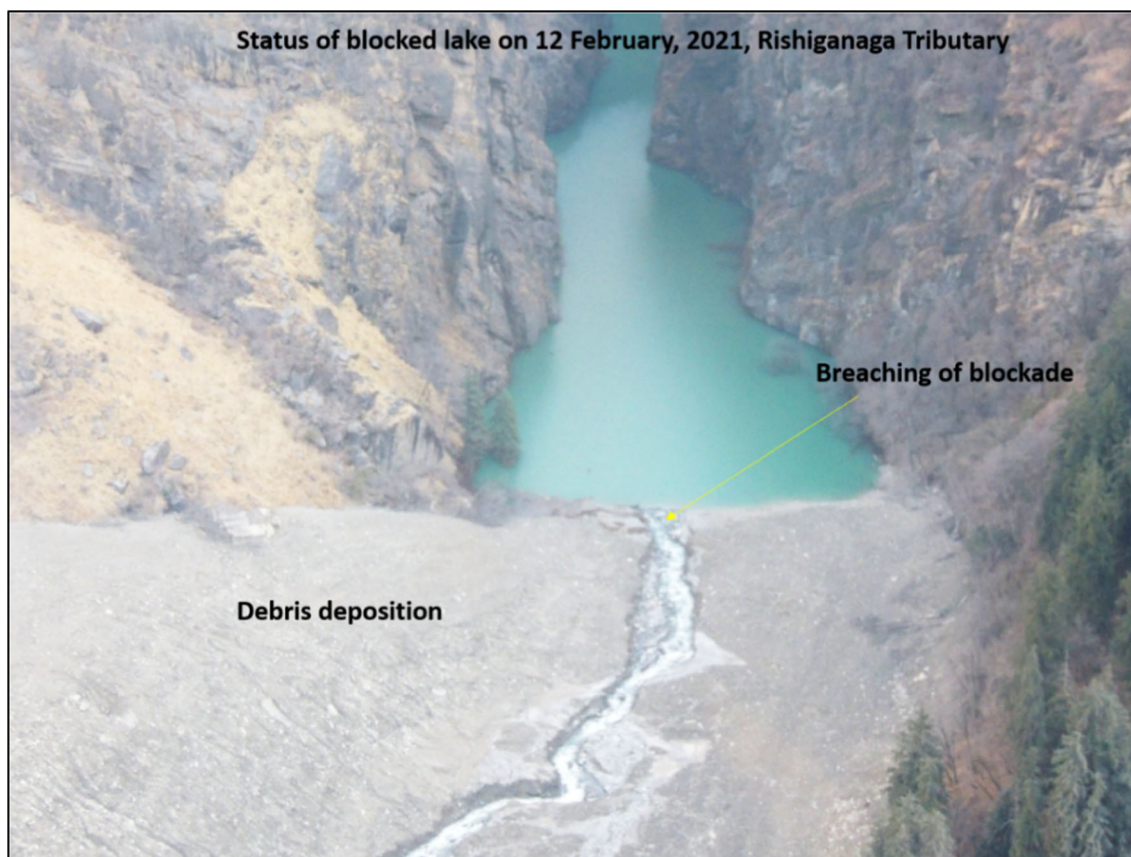
Fig. 7 Aerial photograph (looking toward northeast) of the breaching of the river impoundment (Rishiganga tributary) due to the rockslide in Rishiganga upper catchment
