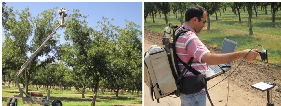
Fig. 1 Left field-level surface reflectance measurements using handheld spectroradiometer, and right instrument calibration using calibrated diffuse white reference panel
