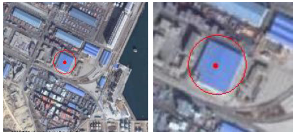
Fig. 6 LoG scale selection operator responses corresponding to two object scales. The extreme location ratio is the scale factor between the objects
