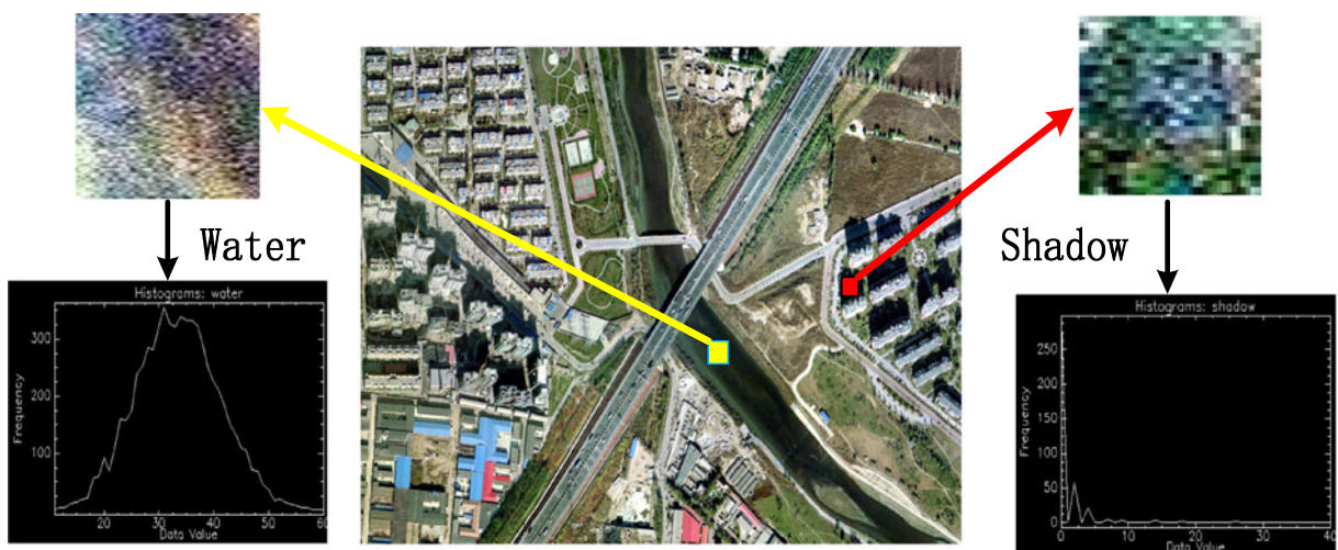
Fig. 7 Histograms comparison of water and shadow
