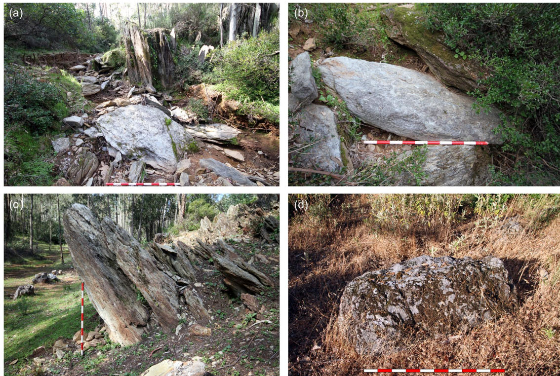
Fig. 12 Types of foliated andesite blocks: detached and in outcrops. a Lenticular block extracted from Quarry 4. b Detached lenticular block in source area 6. c Boudin block from the outcrop of Quarry 1. d Barrel block in the surroundings of Quarry 2
