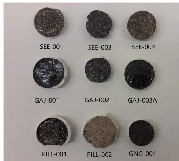
Fig. 3 Raw material samples after heating at 1200 °C for 3 h
