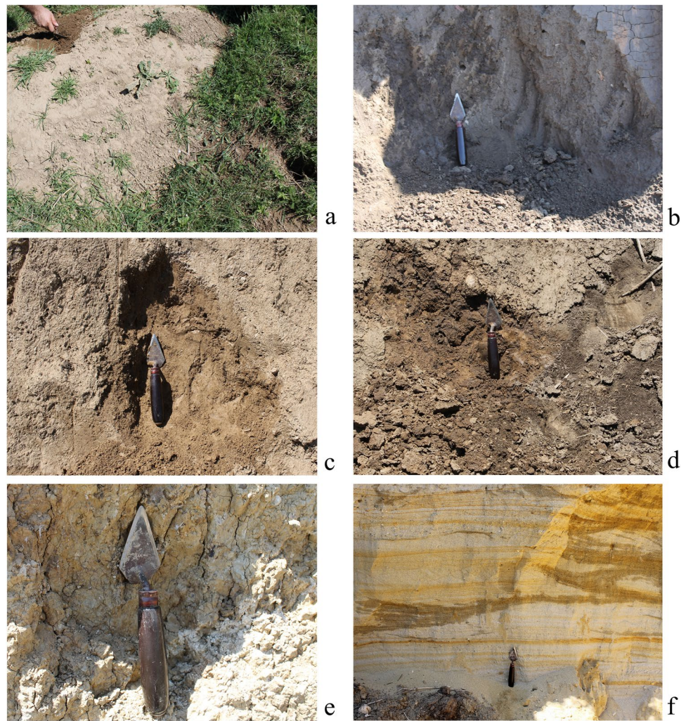
Fig. 4 Pictures showing the outcrops where the geological samples were collected: a GEO 1, very fine sandy clay; b GEO 2, very fine sandy clay; c GEO 3, medium fine sandy clay; d GEO 4, medium fine sandy clay; e GEO 5, coarse sand (created by S. Amicone)
