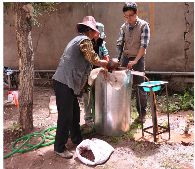
Fig. 8 Flotation machine in 2012, designed and modified from that initially developed by Patty Jo Watson in the 1960s. This is the first time flotation machine is used in archaeology in Tibet
