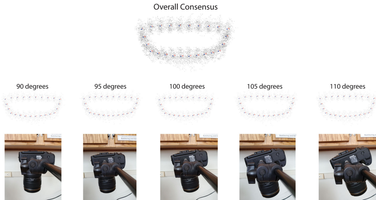
Fig. 3 Consensus configurations for all the imaged microliths with the corresponding camera angles
