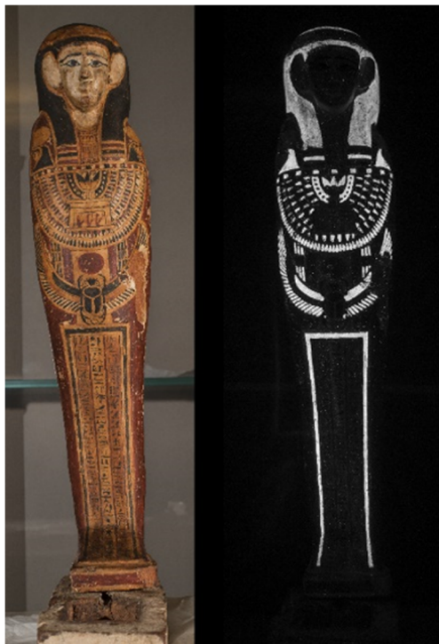
Fig. 1 Visible (left) and visible-induced luminescence (right) images of Ptha-Sokar-Osiris's wooden statue (Ptolemaic era, 332–30 B.C. Cat. N. Provv. 0097, Torino, Museo Egizio). In VIL acquisition, white spots indicate Egyptian blue presence
