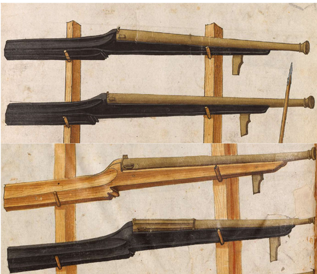
Fig. 5 Heavy brass hackbutts with priming pans on the right side of the breech and with backsights. After Zeugbuch , c. 1502, 72r (top), 72v (bottom). Copyright Bayerische Staatsbibliothek München
