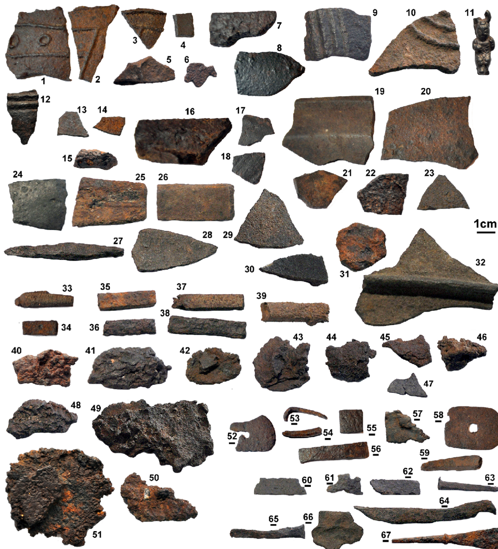
Fig. 2 The general appearance of the iron object under consideration. The numbers identifying the objects are consistent with those in Table 1. The objects were all made of cast iron with the exception of those with the identification number underlined. Objects #33–39 are product intermediaries (Osawa 2005: 45) in the form of square bars excavated from other Mongol sites, often in large quantities (Pohl et al. 2012: 53; Shiraishi and Tsogtbaatar 2009: 559). Objects #40–46 and 48–51 are clearly distinguished by the uniquely irregular surface profile, which is characteristic of a solidification reaction from the partially molten state
