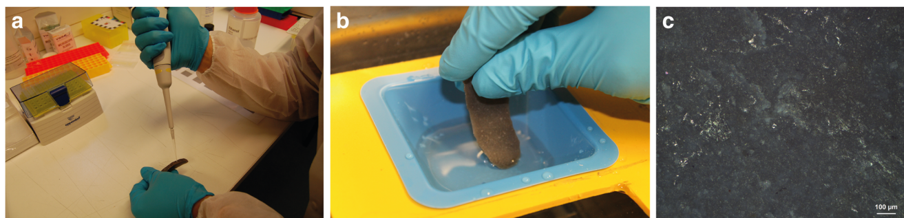
Fig. 1 a Pipette extraction. b Ultrasonic extraction. c Metal residue, extensive polish and striations from using the ultrasonic scaler
