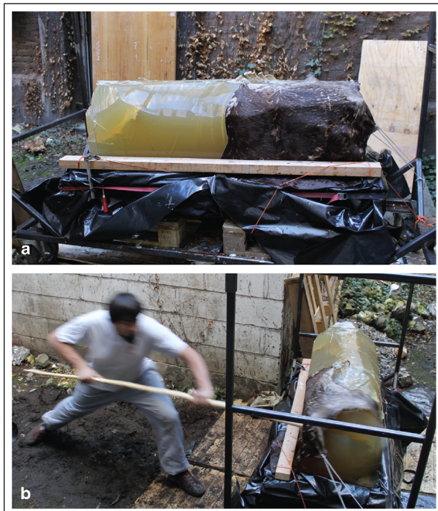
Fig. 10 a Artificial target composed of a bone carcass encased in a ballistic gel, covered with fresh animal hide (after Coppe and Rots, submitted); b experimental tanged tools thrust in the artificial target
