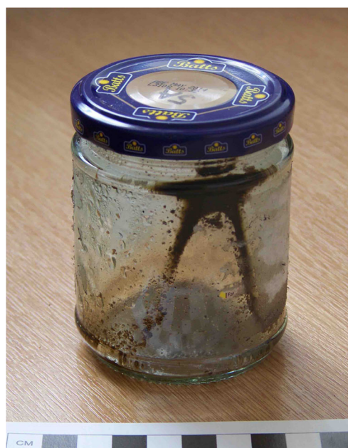
Fig. 11 Tar from mound 5a (5-cm sand cover). The star-shaped pattern on the jar represents the outlet point of the collection tube and resulted from the jar’s almost horizontal position in the ground. This photo was taken 2 weeks after the experiments and some of the viscous tar still clings to the side of the jar
