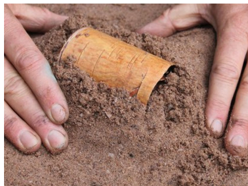
Fig. 1 Experiment 1. Constructing the initial mound of sand that became the model for later experiments 3 to 6. This consisted of placing the 5-cm-diameter roll of the bark flat on the sand then heaping damp sand around it. The mound was built up to the required depth of sand, in this case 5 cm
