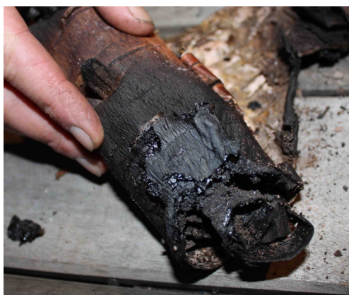
Fig 3 Experiment 1. Roll of bark with charring and traces of tar
