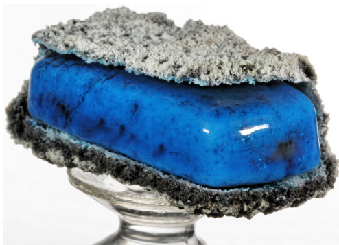
Fig. 6 Faience object surrounded by its capsule (BR body paste, glazed by the GP11 glazing mixture)
