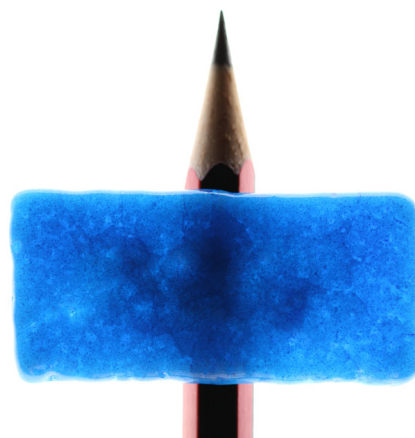
Fig. 7 Translucent faience object (about 6.5 mm in thickness) produced by the GP11 glazing mixture and the B2 body paste
