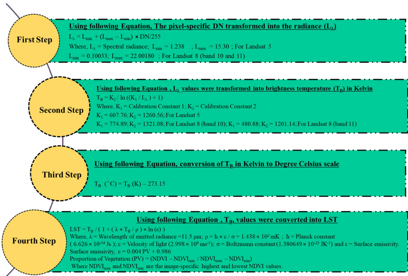
Fig. 2 Process of seasonal LST estimation using Landsat thermal bands
