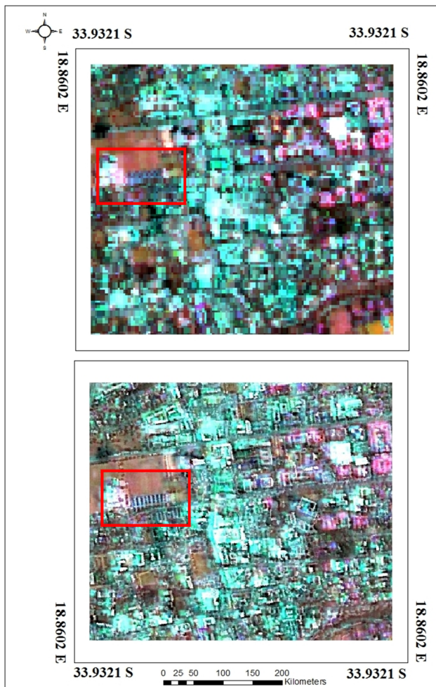
Fig. 6 Top: original SPOT5 10 m multispectral image and at the bottom the resolution merged image
