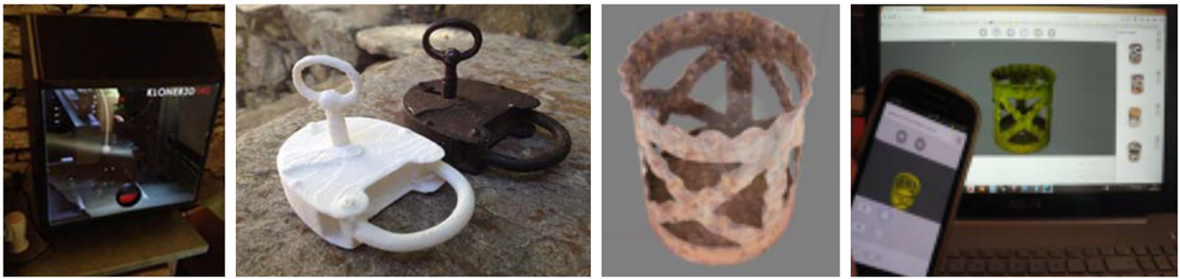
Fig. 8 Starting from the left: (i) 3d printing of photogrammetric models; (ii) the real object and its printed copy; (iii) and (iv) sharing high-resolution 3d models of small objects in an online visualisation system (BIM3DSG)
