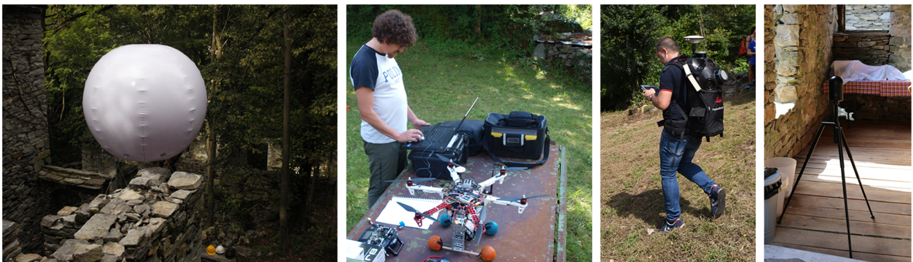
Fig. 2 Starting from the left: (i) tethered balloon; (ii) UAV; (iii) Leica Pegasus Backpack; (iv) Leica BLK360
