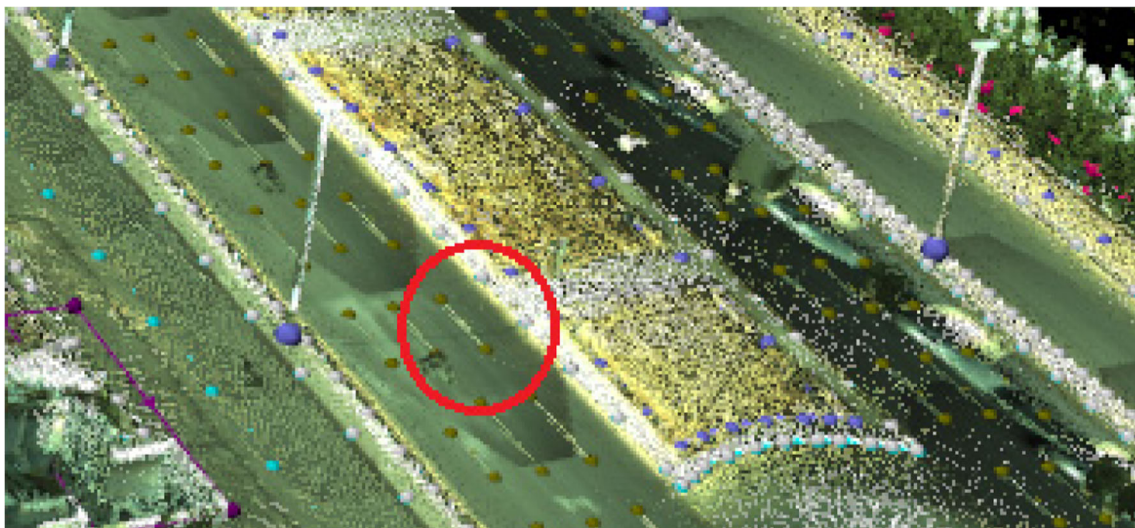
Fig. 11 Point cloud and road markings extraction
