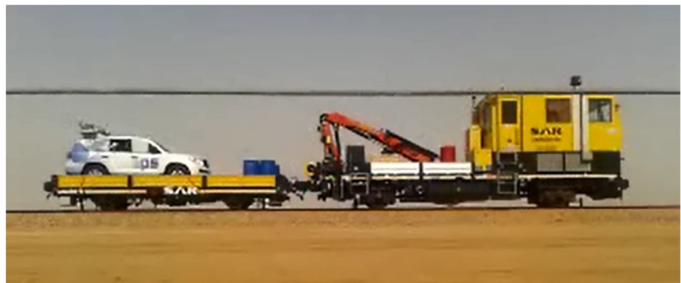
Fig. 7 Railway survey using the LYNX MMS
