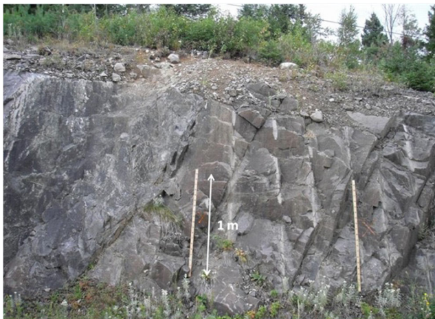
Fig. 3 Outcrop of fractured crystalline bedrock (anorthosite) in the Saguenay-Lac-St-Jean region located in Quebec, Canada (after Chesnaux 2013)
