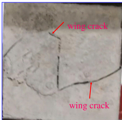
Fig. 7 Wing crack of the specimen when the crack length is 40 mm and the crack dip angle is 90°
