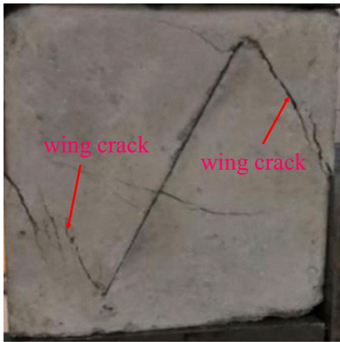
Fig. 13 Wing crack of the specimen when the crack dip angle is 60° and the crack length is 80 mm
