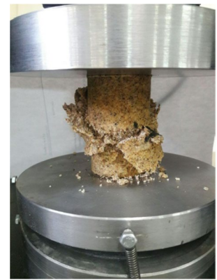
Fig. 9 Specimen collapse and shearing paths failure
