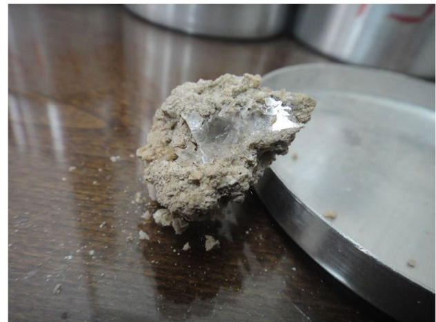
Fig. 4 A sample of gravel and finer sized gypsum crystal particles found in the site soil
