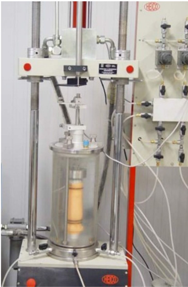
Fig. 4 Triaxial test equipment is used in this study
