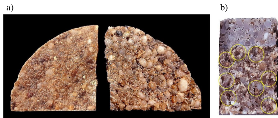
Fig. 9 a View of specimens with high and low resin contents (left: an H series specimen and right: an L series specimen), b fractured surface of an L series specimen and the air voids
