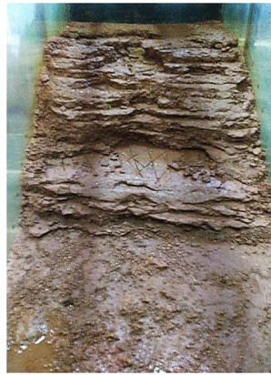
Fig. 10 Rill erosion observed in 30° slope
