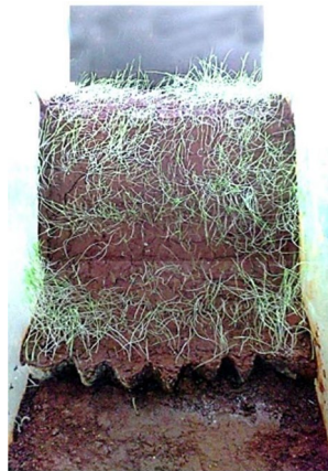
Fig. 18 View of bamboo geocell protected 60° slope at different durations of heavy rainfall, (a) Bamboo geocell protected 60° slope at 0 min 0 s, (b) Bamboo geocell protected 60° slope at 253 min 54 s, (c) Bamboo geocell protected 60° slope at 837 min 54 s
