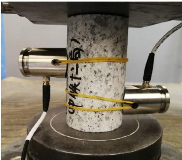
Fig. 6 Installation of AE sensors
