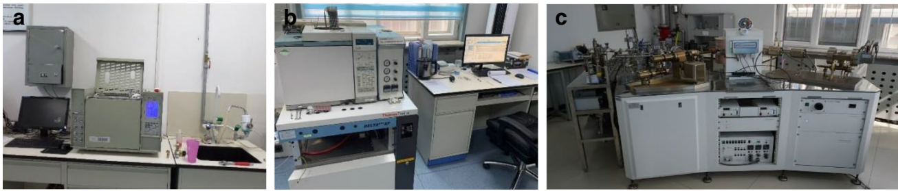
Fig. 1 The test instruments for component content and isotope values. a Agilent 6890 N. b Delta Plus XP. c Noblesse
