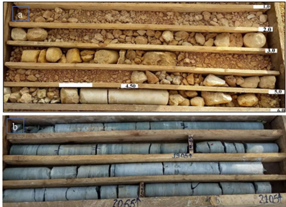
Fig. 5 Selected core samples from Chalchal dam site: a sandstone rock unit (BH4, depth interval: 1.00–6.00 m), b massive limestone rock unit (BH1, depth interval: 17.85–21.05 m)
