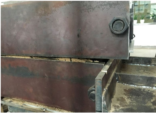
Fig. 6 The gap between boxes during shearing process under 400 kPa normal stress ( RS800* )
