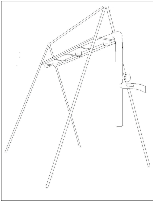
Fig. 3 Pressurized rainfall simulator
