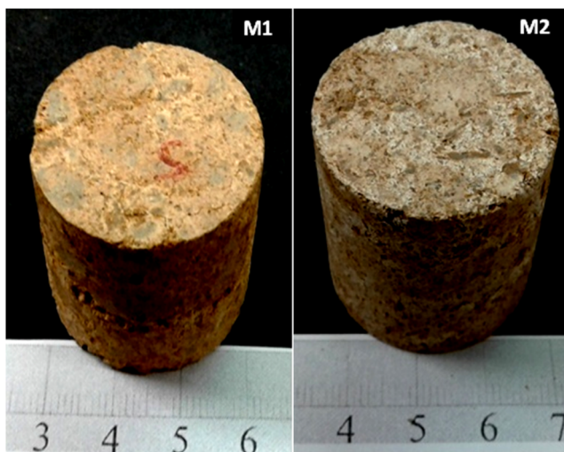
Fig. 9 The refractory specimens elaborated using mixtures M1 and M2
