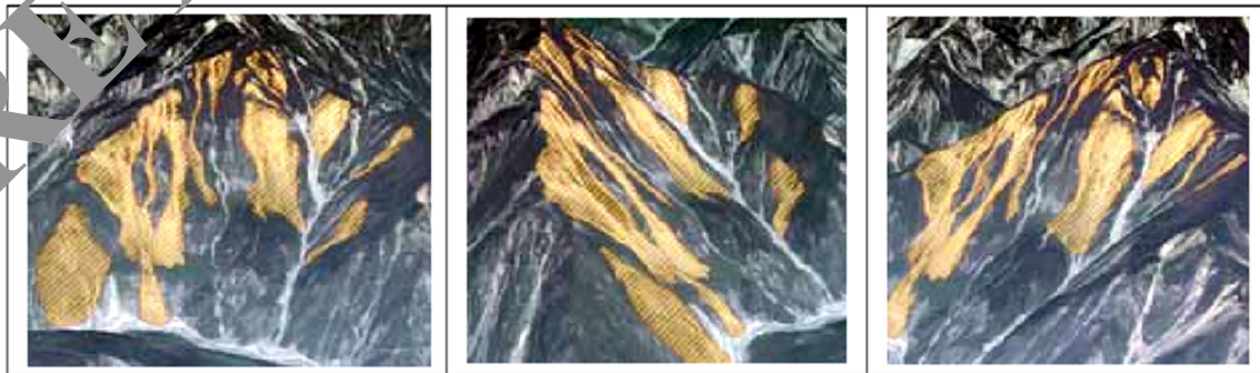
Fig. 3 Interpretation under the three-dimensional view of the landslide (from left to right as the front, left side, and right side)
